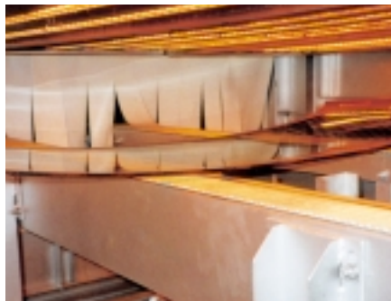
Preheating of glass prior to application of PU foam
