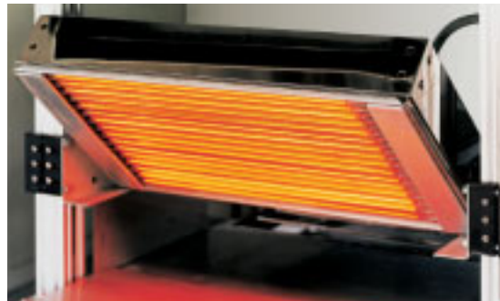
Carbon IR emitter array testing in the Application Centre at Heraeus Noblelight
